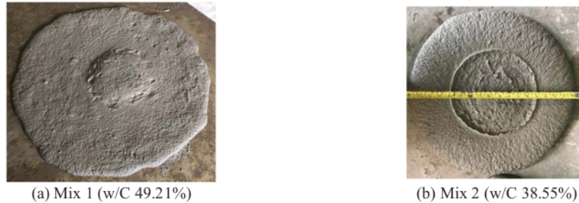
FIGURE 2. Flowability of fresh foam concrete
